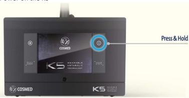
Note: After power on, the K5 sampling pump is always active to ensure optimal warm-up time (sampling pump goes into a 2 min standby when any command on screen is selected).
