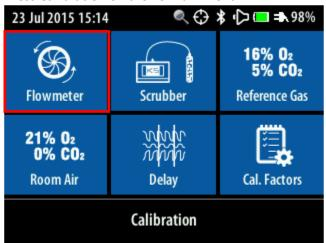
Press **Flowmeter** and follow the instructions on the screen – fill and empty the 3-litre syringe completely at various speed.
