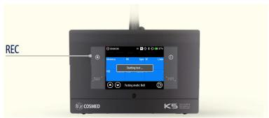
Press the **REC** button to start the recording but recommended to wait approx. 1 minute to flush internal chambers.
