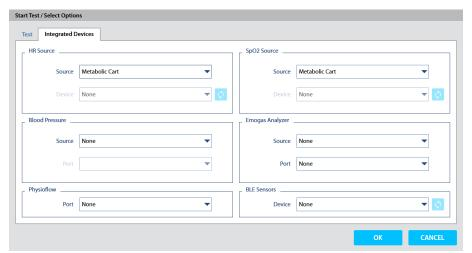
On tab **Integrated Devices** select **HR Source** to "Metabolic Cart", if HR is coming from ANT+ or Bluetooth receiver inside K5.
