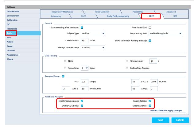
O2 kinetics: If exercise is performed as a step test, the response of the VO2 can be analysed.
