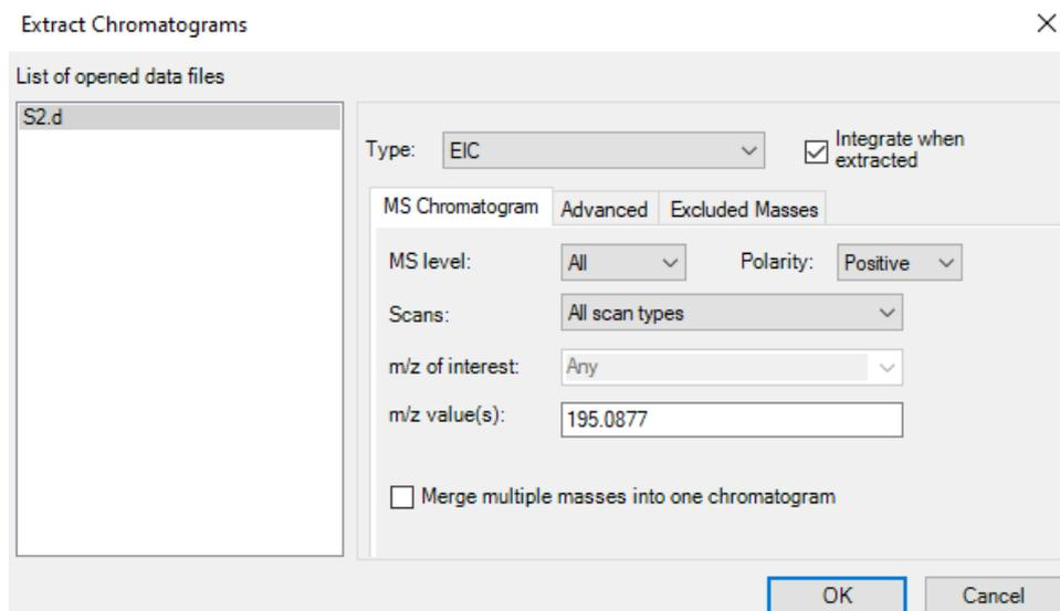
If an ion with similar  $m/z$  is found, you will see its retention time in extracted ion chromatogram. Right click on top of the chromatogram and choose Smooth chromatogram. Then from smoothed chromatogram extract the MS spectrum and see if your compound can be found in the spectrum.
