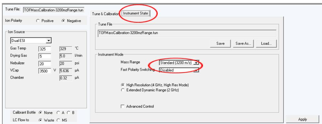
In *Tune & Calibration*, choose the polarities where you want to calibrate (positive, negative or both) choose Mass Calibration/Check and press Start TOF Mass Calibration. After calibration Tune reports are displayed.
