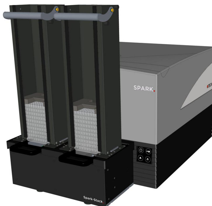
Figure 85: The built-in Spark-Stack microplate stacker for automated loading, unloading and restacking of up to 50 plates per run.
