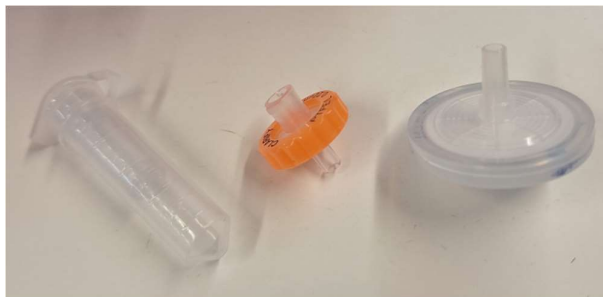
Figure 4. Different filters. Left: spin filter, Middle and right: two different syringe filters.
