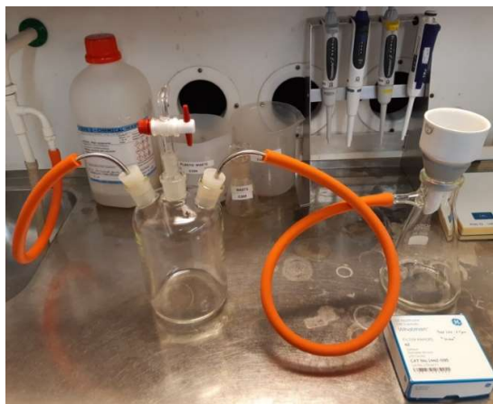
Fig.5. Buffer Filtration system.
