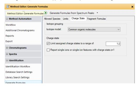
Make sure the correct spectrum is chosen active, and press Generate Formulas from Spectrum Peaks.
