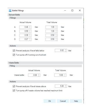
D before use. Right click on top of Quat Pump icon → Prepare pump. Choose the line that you wish to purge by changing its composition to 100%, then purge that line 5 minutes with the rate of 5 ml/min by pressing start.
