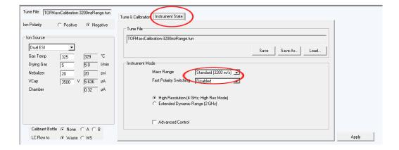
In *Tune & Calibration*, choose the polarities where you want to calibrate (positive, negative or both) choose Mass Calibration/Check and press Start TOF Mass Calibration. After calibration Tune reports are displayed.
