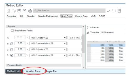
In Worklist, create a new list (or open your former modified list) and add your sample(s) to the list. Place the vials to the multisampler and add the locations to the list accordingly. The locations have to be in form P1-A1 (P1 = plate 1 or 2, A1 = coordinate of your sample in the plate). If there are old samples inside multisampler, place them to measured MS samples tray on the table.
