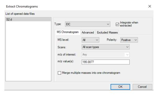
If an ion with similar m/z is found, you will see its retention time in extracted ion chromatogram. Right click on top of the chromatogram and choose Smooth chromatogram. Then from smoothed chromatogram extract the MS spectrum and see if your compound can be found in the spectrum.
