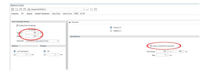
After this turn the UV lamp on from VWD. Right click on top of the icon, and choose switch on. The UV-lamp needs to warm up for ~15-20 minutes before the runs.
