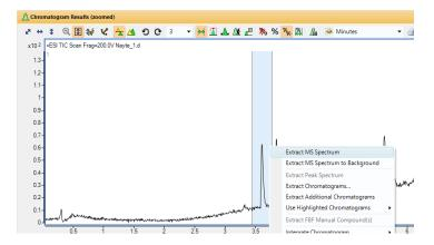
Analyse the spectrum. If you observe your compound, you can generate the accurate mass report. To get the report for accurate mass, open from the method editor (down on the left) Data\_Analysis\_Qual method.
