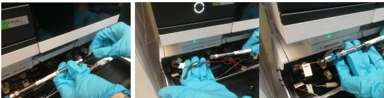
Opening the connector, quick connector (left), connector with handle open (middle), handle closed (right)
